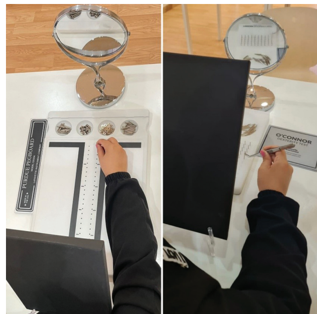
Fig. 2 Purdue Pegboard Test and O'Connor Tweezer Dexterity Test using indirect vision.
